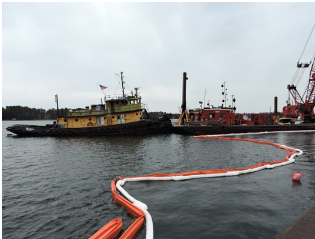
Graham Jaehnig/Daily Mining Gazette Containment booms surround leaking petroleum from the sunken Katherine while a recovery barge and the tug Jean C. raise the Dawn Tuesday in the Lower Entry.
